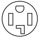
4-wire receptacle (14-30R)
