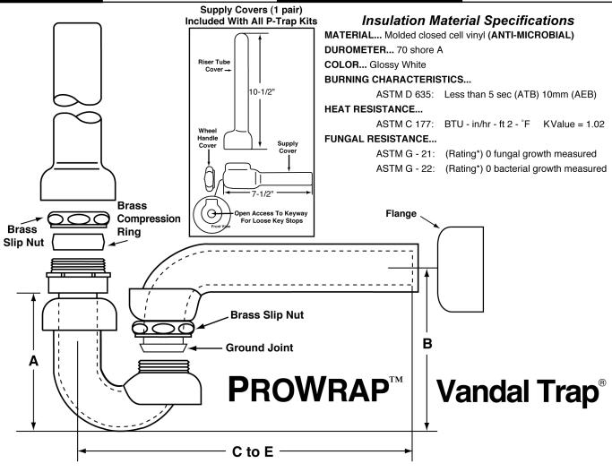
\*ASTM Rating - Observed Growth on Specimens
