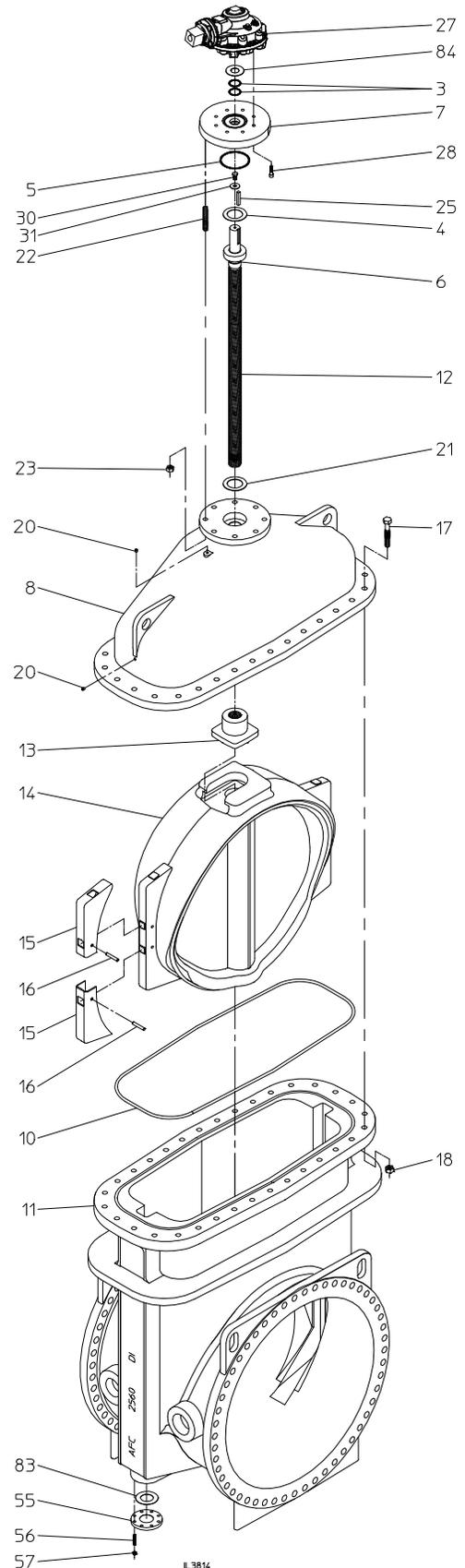
\*\* On horizontal configurations, the blind flange (Ref. # 55) will be located on the bottom of the valve guide track, opposite the direction in which the bevel gear input shaft is installed.
