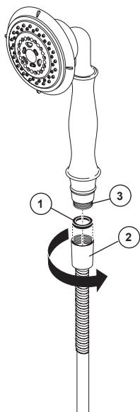
Seat the gasket (1) firmly into the hose nut (2). Carefully align the thread of the tapered end of the hose nut directly to the hand shower (3). **Hand Tighten—do not use a wrench or pliers.** Then place the hand shower into the wall mount holder (4).
