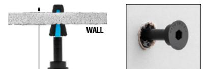
6. Secure WINGIT and Accessory with the enclosed 3.5" Stainless Steel Screw
