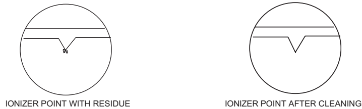
Fig. 19. Removal of deposits from ionization points.
