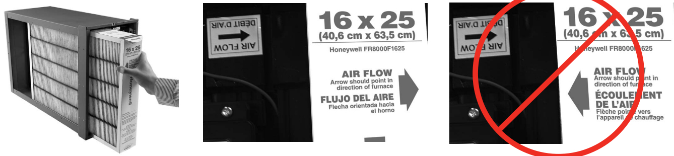
Fig. 18: Make sure that the arrows on the filter point in the same direction as the arrow on the enhancement module. This will be in the same direction as airflow.
