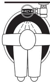
3. Once a user is detected, if the user leaves in 65 seconds or less, a reduced flush will automatically initiate. The circuit automatically resets and is ready for the next user.
