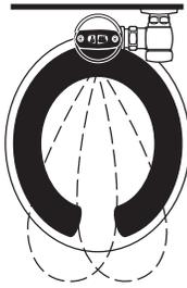
2. As the user enters the beam's effective range, 22" - 42" (559 mm to 1067 mm), the beam is reflected into the Scanner Window to activate the Output Circuit. Once activated, the Output Circuit continues in a "hold" mode for as long as the user remains within the effective range of the sensor. If the user stays longer than 65 seconds, a full flush will automatically initiate when the user leaves.
