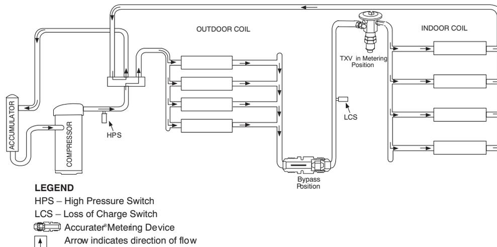
**Fig. 17 - Typical Heat Pump Operation, Cooling Mode**
