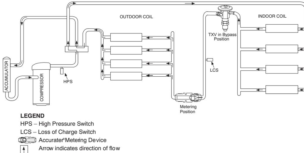
Fig. 19 - Typical Heat Pump Operation, Heating Mode
