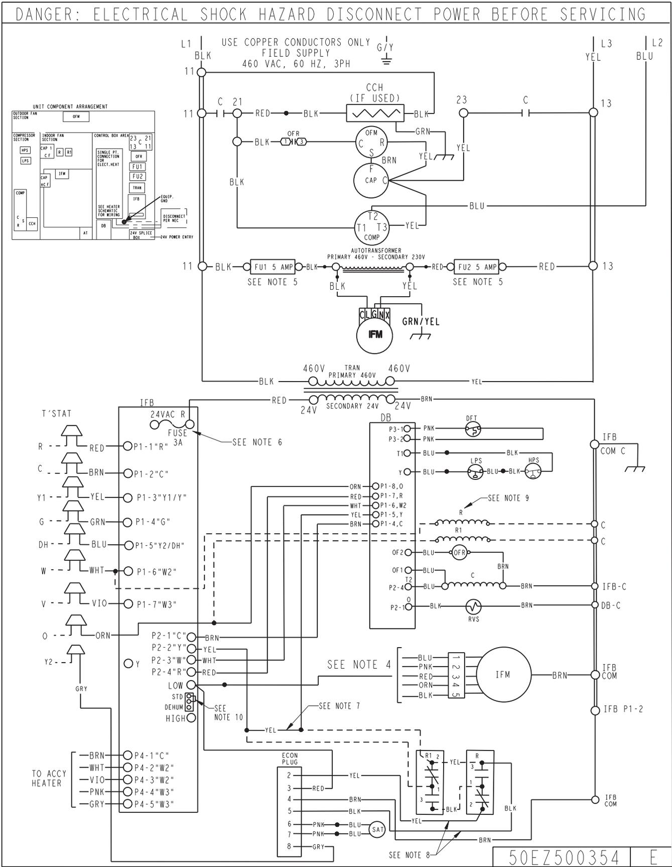
Fig. 14 Cont. - Ladder Wiring Diagram 460-3-60
