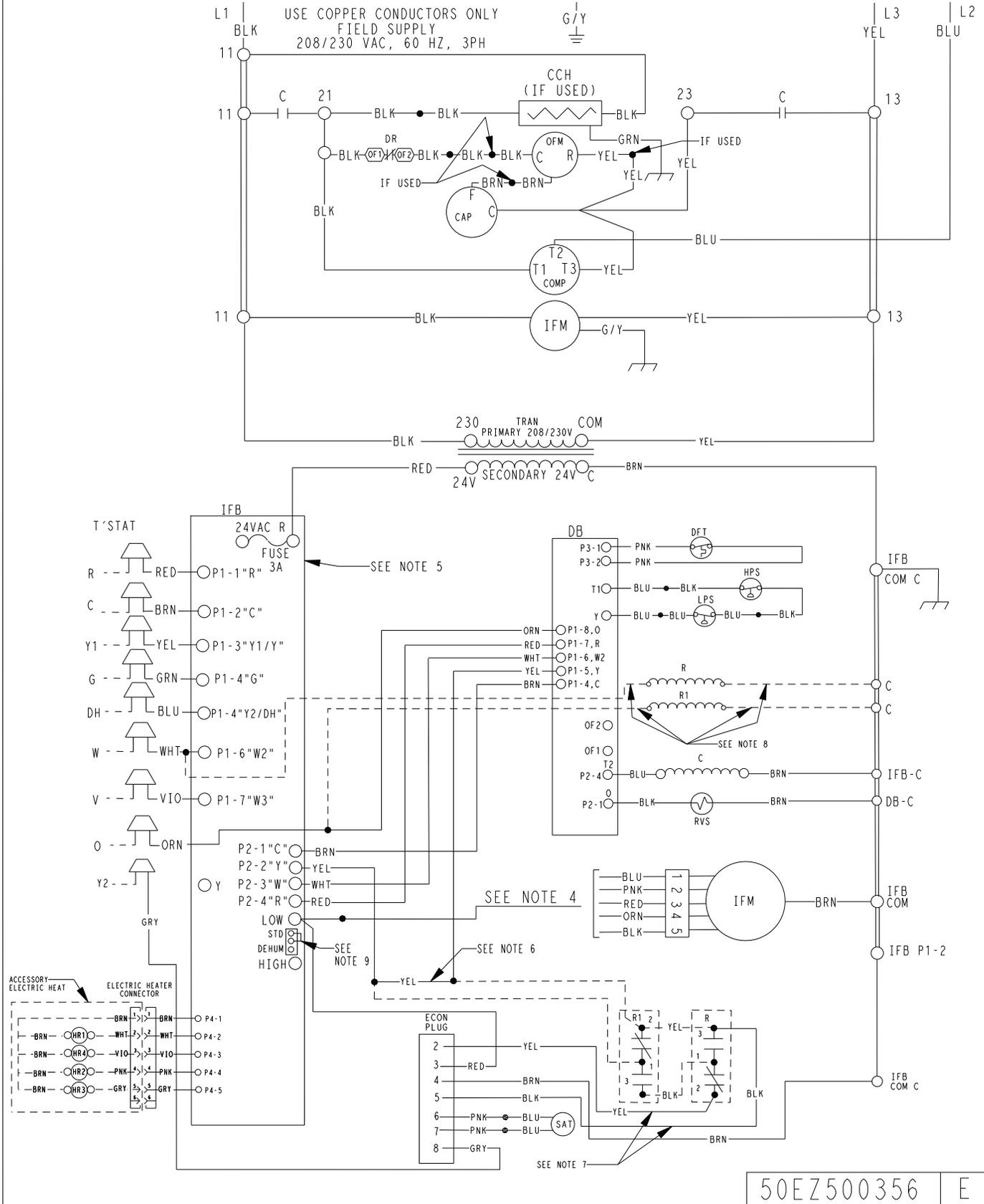
Fig. 13 Cont. - Ladder Wiring Schematics - 208/230-3-60
