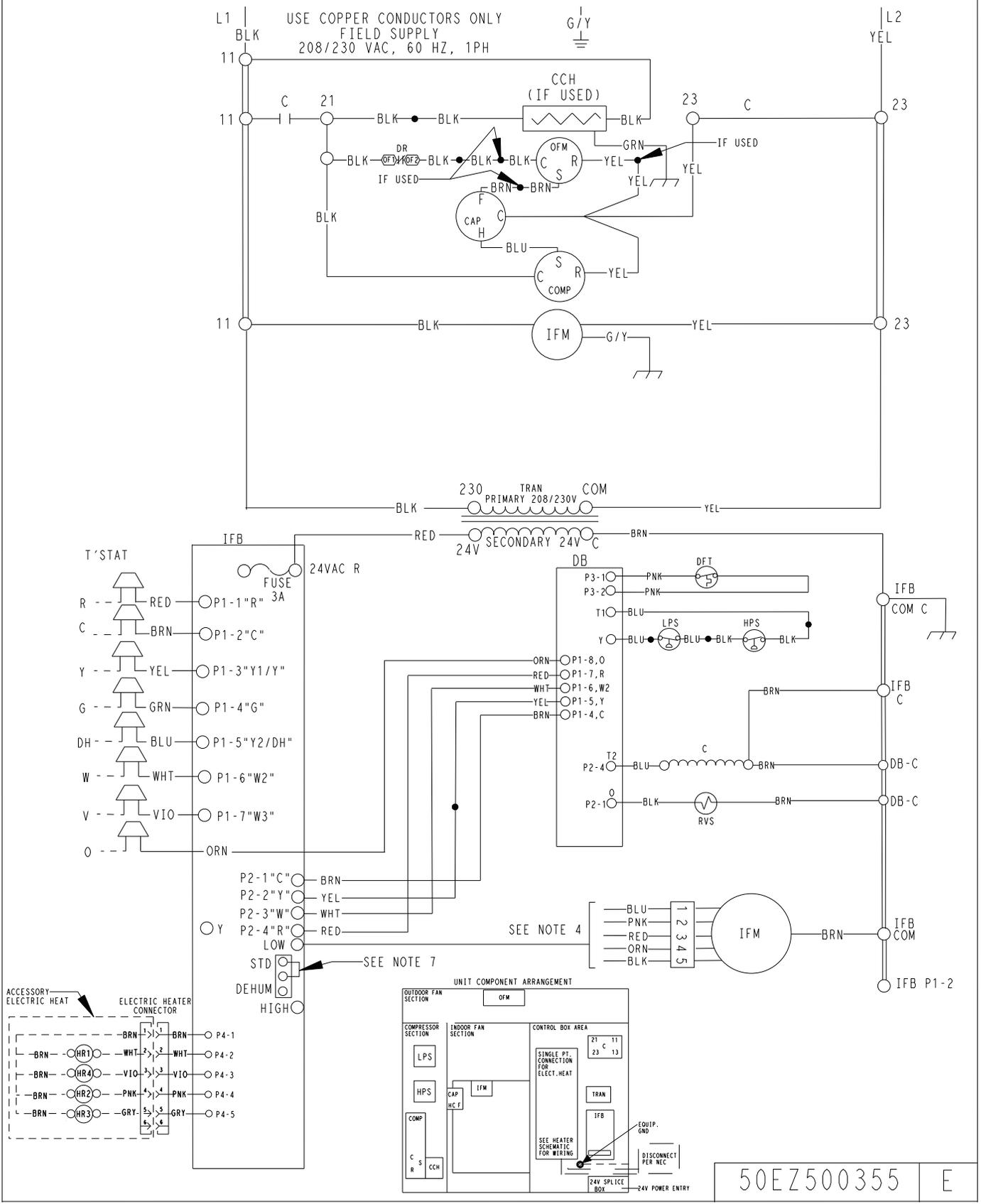
Fig. 12 Cont. - Ladder Wiring Schematics 208/230-1-60
