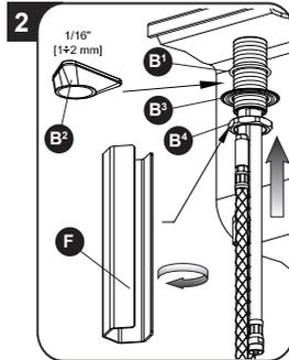
For countertop thicknesses less than 1/16" thick use the rubber gasket (B1) and mounting flange (B2), for all other installations use the rubber gasket (B1) and metal washer (B3). Secure mounting hardware in place by tightening mounting nut (B4) with wrench (F).
