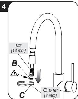
4 Unscrew the bushing connected to the end of the hose (B) paying attention not to lose the rubber gasket (C).
