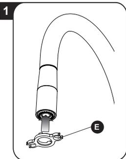
1 Before removing the aerator make sure that the faucet is turned off. Unscrew the aerator using the aerator installation key (E) included with the faucet. If the aerator is clogged just rinse it with running water. Do not use detergents. Reassemble the aerator by following the instructions in reverse order.
