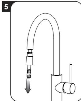
5 You can now totally remove the hose from the faucet body and replace it with a new hose. Reassemble the hand shower assembly by following the instructions in reverse order.
