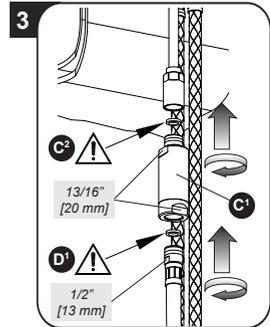
Install the check valve (C2) to the outlet hose with a rubber washer (C1). Secure with wrench. Attach the pull-down hose to the bottom of the check valve with a rubber washer (D1). Secure with wrench.
