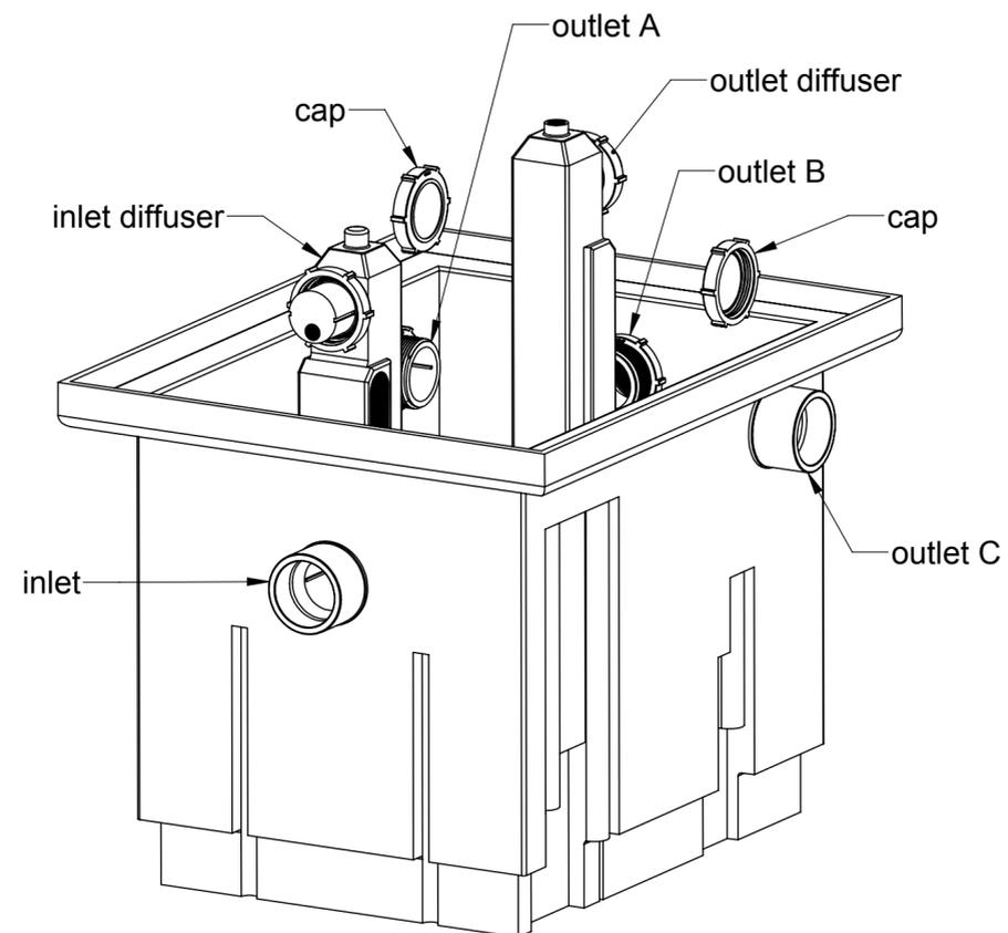
Schier grease interceptors are rated and manufactured with an internal flow control system already in place. They do not require an external flow control fitting.
