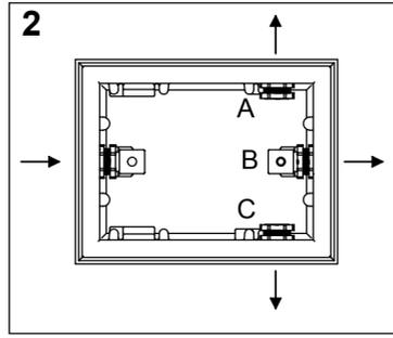
2 Connect outlet diffuser to the desired outlet (A, B or C). Unit is shipped with outlet diffuser in location B.
