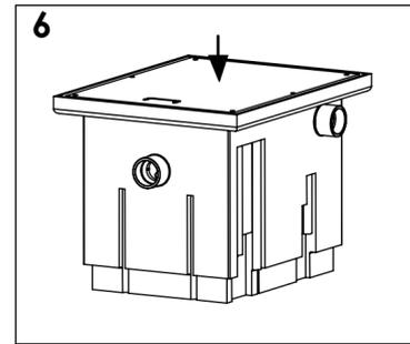
6 Run sinks to fill unit and replace cover.
