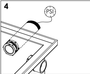
4 To conduct a pressure test on the pipes, remove diffusers and fasten green caps to the inlet and outlet connections. Do not pressure test unit.
