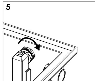
5 Hand tighten inlet/outlet diffusers and caps back to chosen positions.
