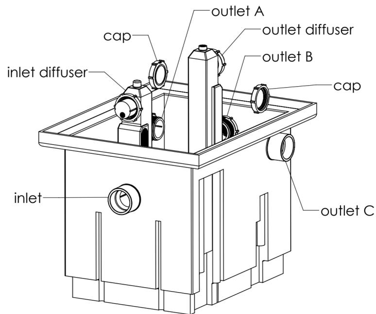
Schier grease interceptors are rated and manufactured with an internal flow control system already in place. They do not require an external flow control fitting.
