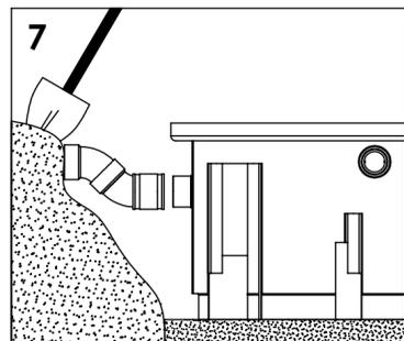
7 If unit is buried, backfill with sand or pea gravel. Pour concrete and install finished floor. Roll down inlet line using (2) 45° elbows immediately preceding the unit to ensure inlet pipe is clear of water. **Note: Maximum extension dimension is 36"**
