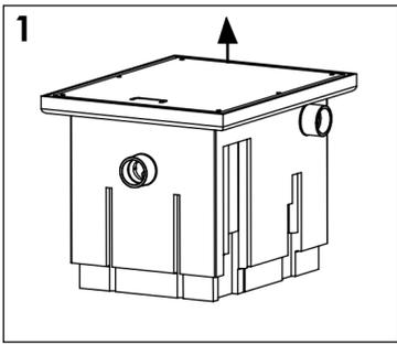
1 Set unit on level and solid surface near the sink. Remove cover.
