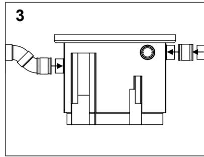
3 Connect inlet and outlet pipes to unit. Roll down inlet line using (2) 45° elbows immediately preceding the unit to ensure inlet pipe is clear of water.
