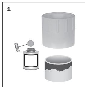
Glue adapter to pipe using appropriate solvent cement.
