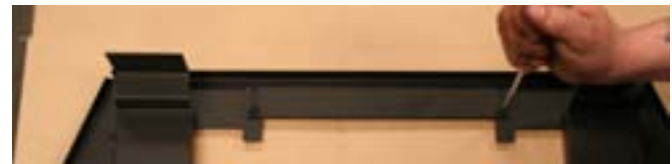
Figure 8c. Pull the air baffle forward as far as possible and screw the air baffle closed.
