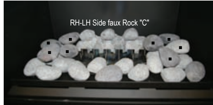
Figure 28c. Placement of (8) eight LH & RH Side "C" faux ceramic rocks. (Marked). Note: approximate location and placement. (Place on top, in between the lower layer rocks in a pleasing pattern).
