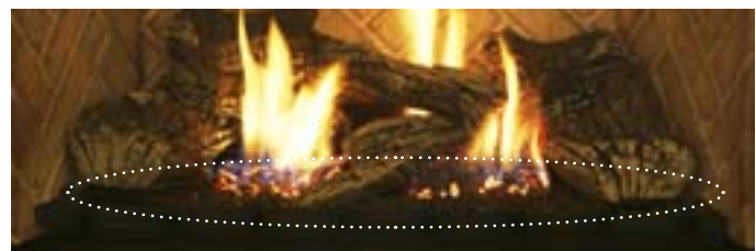
Figure 29e. Ember placement, (fill voids between front logs and along the front of the grate / pan).
