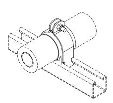
THE HOLDRITE<sup>®</sup> Insulation Coupling "7 Series" strut clamps are for use with insulated pipe lines mounted to strut in any orientation. These are plenum rated insulation clamps are ideal for insulated pipe line support without the need for rigid insulation supports or insulation shields.
