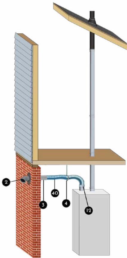
**BlitzFlex®** Sidewall Termination, where **BlitzFlex®** provides one continuous air-intake from appliance adaptor to termination, and terminates horizontally with a **Centrotherm BlitzKit**.
