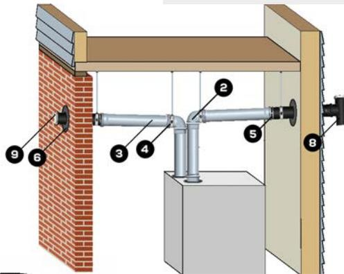
InnoFlue® SW side wall installations, where exhaust and air supply remain separated through the Low Profile Wall Termination.
