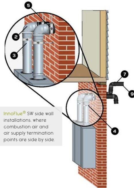
InnoFlue® SW side wall installations, where combustion air and air supply termination points are side by side.
