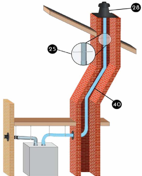
**BlitzFlex®** is designed to handle offsets in your air-intake run, and will reduce necessary components thus saving you time and money on every job. Uncoil **BlitzFlex®**, cut to length, and install a continuous in-take system in minutes. Additional supports may be required on longer runs.
