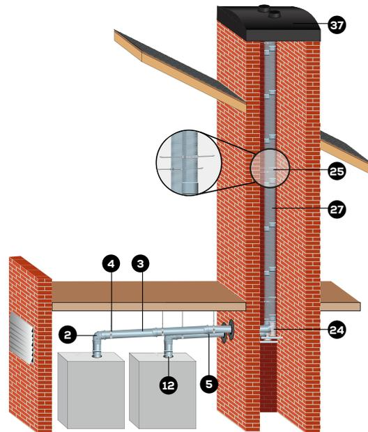
InnoFlue® SW and Flex installations, where InnoFlue® SW is used to pass flue gases to the base of the chimney, then InnoFlue® Flex to get them to the termination at the top. Combustion air is not supplied through the masonry chimney.
