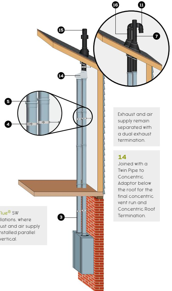
Exhaust and air supply remain separated with a dual exhaust termination.
