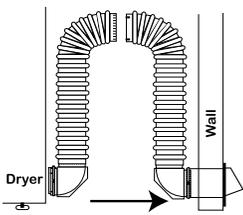
Guide dryer into position. Joints on elbows swivel to allow motion.
