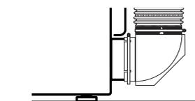
To connect the elbow to the dryer, position a clamp so that it covers the slot in the elbow. Slide the elbow over the dryer exhaust pipe. Tighten clamp.
