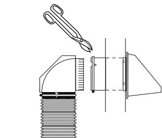
When connecting to a wall pipe, cut a 1" long slit in tailpipe. Position a clamp so it covers the slit in the vent tailpipe. Insert crimped fitting into tailpipe. Tighten clamp.
