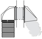
Check installation by inspecting airflow outside. Verify hood flapper is pushed fully open when the dryer is turned on.
