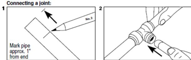
Push the pipe and fitting together firmly with a twisting action until it clicks. Allow at least 1" clearance between fittings for disconnection.
