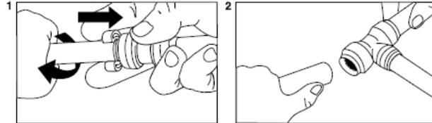
Push the disconnect clip against the release collar and pull the pipe with a twisting action.
