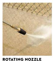
5100 PSI Rotating zero-degree nozzle for aggressive cleaning of stubborn stains.
