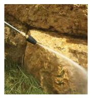
**ROTATING NOZZLE 3000 PSI** Rotating zero-degree nozzle for aggressive cleaning of
