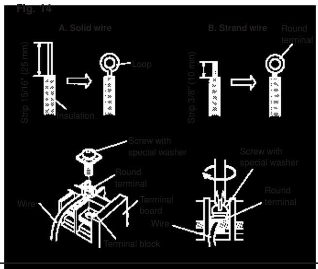
**(1) Match the terminal block numbers and connection cord colors with those of the outdoor unit. Erroneous wiring may cause burning of the electric parts.**
