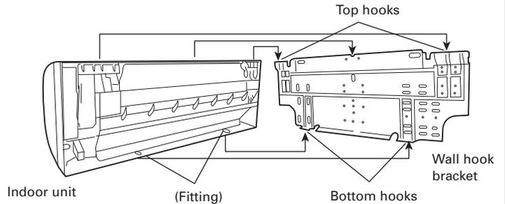
After hooking the indoor unit to the top hook, hook the fittings of the indoor unit to the two bottom hooks while lowering the unit and pushing it against the wall.
