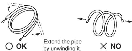
Do not bend the pipes in an angle more than 90°. When pipes are repeatedly bent or stretched, the material will harden, making it difficult to bend or stretch them any more. Do not bend or stretch the pipes more than three times.
