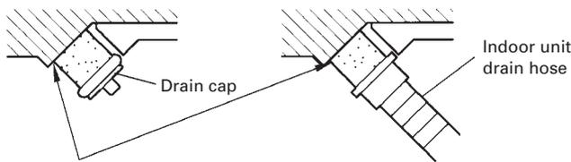
Insert the drain cap and drain hose until it butts against the drain port.
