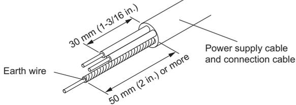
How to connect wiring to the terminal
