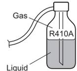
Add refrigerant from the charging valve after the completion of the work.
