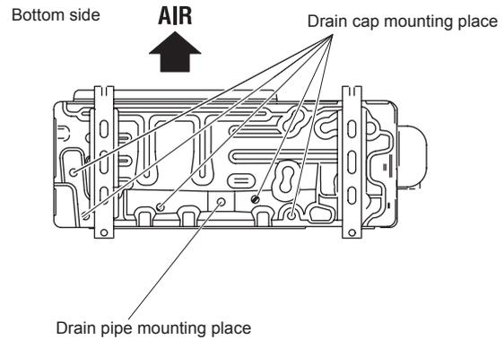
Since the drain water flows out of the outdoor unit during heating operation, install the drain pipe and connect it to a commercial 16 mm hose. (Reverse cycle model only)
