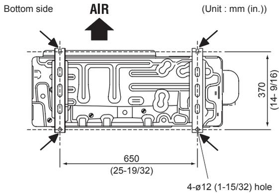
Fix securely with bolts on a solid block. (Use 4 sets of commercially available M10 bolt, nut and washer.)
