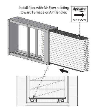
Align filter in top and bottom rails and slide into place. Reinstall door.
