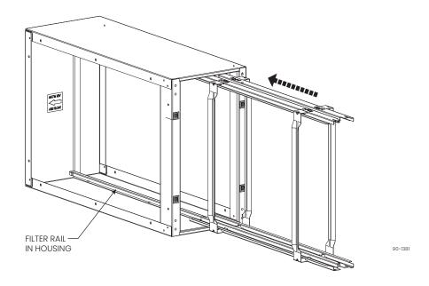
**5.** Secure the metal rail system to the outer housing using four 1/2" long sheet metal screws.
