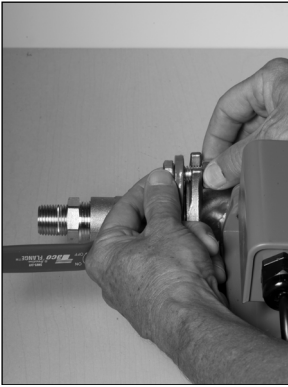
3. Attach shut-off flanges to pump.
