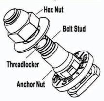
Now when the "Hex Nut" turns so does the "Bolt Stud". With each turn the "Bolt Stud" becomes shorter as it threads down into the "Anchor Nut".
