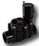
Heavy duty construction with stainless steel screws. External bleed to manually flush system. Operate manually or automatically. Used in conjunction with a back flow preventer. CP Valve is same as DV valve on commercial side.
