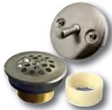
Trip Lever bathtub tub drain overflow conversion kit includes: 2-hole trip face plate with handle, 2 screws, tub drain shoe with a plastic adapter to fit 1-1/4"-16 or 1-1/2"-11 threaded waste elbow. Will fit most manufacturers tub waste and overflows.
