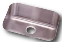
Formed of nickel bearing stainless steel. Fully undercoated to dampen sound and prevent condensation. Bowl size: 21" x 15-3/4" x 8". Minimum cabinet size 27". Limited lifetime warranty.
