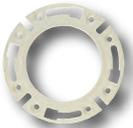
Build up existing flange when added subfloor, tile, etc. leaves flange at or below floor level. Sits on top of existing ring adding 7/16" height.
