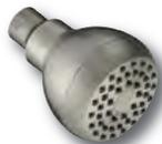
2-3/4" Face, solid brass swivel connection, 1.5 GPM flow rate, single-function shower head. Easy clean rubber nozzles, Qualifies for LEED points, Uses 40% less water than conventional 2.5 GPM shower heads, WaterSense® certified.
