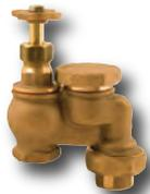
Yellow brass construction, import valve. Atmospheric vacuum breaker prevents the back flow of irrigation system water into the household supply. Full size waterway for low pressure 25 to 150 P.S.I.
