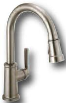
Maximum 1.5 GPM @ 60 psi, 5.7 L/min @ 414 kPa. One, two, three, four hole mount options (escutcheon and soap dispenser optional, sold separately). Two-function wand; aerated stream or spray. Dual integral check valves in sprayer. Ceramic cartridge. Spout rotates 360°. Red/Blue indicator markings. Polymer braided flexible supply hose with with 3/8" compression fitting - 28 7/8" (733mm) long.
