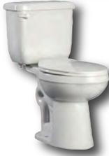
1.28 GPF, High Efficiency Toilet. Two-piece vitreous china. 2" fully glazed trapway. Anti-siphon fill valve. Gravity fed, box rim. Close coupled tank with cover. Elongated skirted bowl, 16-1/2" height. PF5112NHEWH tank with chrome flush lever. PF5112HEWH tank with color match flush lever. EPA WaterSense compliant. Meets ANSI ASME A112.19.2-2013-CSA\_B45.-13.
