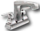
DIAMOND Seal® Technology. Maximum 1.2 GPM @ 60 psi, 4.54 L/min @ 414 kPa. Three hole mount. Diamond coated ceramic cartridge. 3/8" O.D. straight PEX supply lines. Models without "TP" suffix have metal drain with pop-up type fitting with plated flange and stopper. Models with "TP" suffix have polypropylene pop-up type drain fitting with plated metal flange and stopper cap. Optional thick deck kit (RP76691) adds 1-1/4" max. deck thickness.
