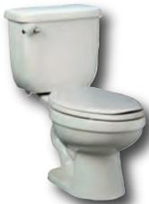
Ultra high efficiency toilet. 1-3/4" fully glazed trapway. Gravity fed. Anti-siphon fill valve. Close coupled tank with cover. Quick connect 2-bolt tank to bowl installation. Color matching trip lever. 3" Flush valve. Sanitary bar on all bowls. Available round front and ADA elongated. EPA WaterSense Certified. One-Year limited warranty.
