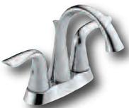
Diamond coated ceramic disc cartridges. 3-hole installation. 4" centerset. Includes metal pop-up assembly. 1.5 GPM flow rate at 60 PSI. EPA WaterSense approved. CAL Green compliant. ADA compliant. Lifetime warranty.
