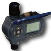
EVO 100i is a Hose End Timer with a 3/4" female thread inlet and male thread outlet and fueled by the surrounding ambient light (solar). After being charged, this efficient energy system provides enough power for the timer to function at any time, night or day, and in any weather with no direct sunlight or batteries required. Run times from 1 minute up to 6 hour. 5 start times can be used a specific days of week, odd or even. Simple start programming.
