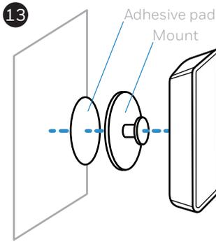
Before mounting, check to make sure surface is clean enough to ensure good adhesion.
