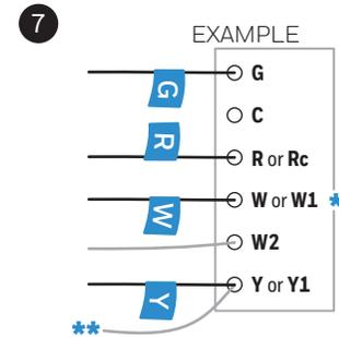
Use the provided stickers to label the following connected wires:
