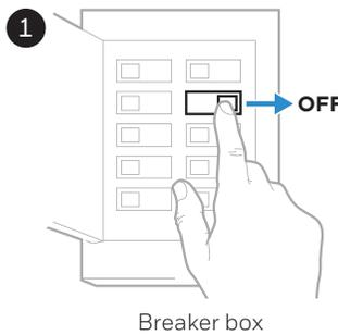
Turn the power off at the breaker box or control switch for your HVAC\* system.
