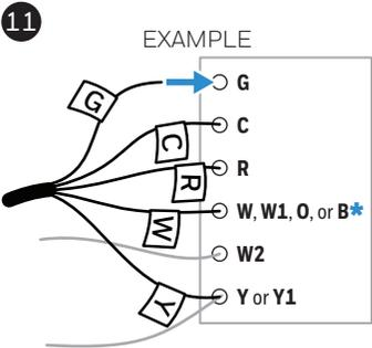
Connect the wires from the "Equipment" labelled side of the C Wire Adapter to the matching terminals on the control board.
