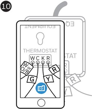
Take a picture of the wires you inserted into the C Wire Adapter.
