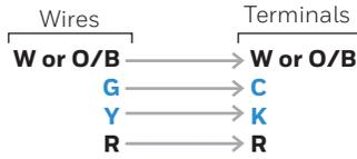
This will convert the G and Y-wires into C and K-wires.
