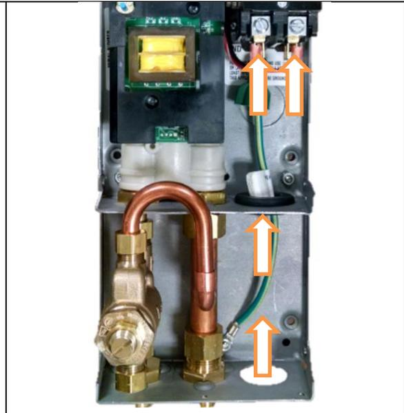
2) The power leads are to be secured to the L1 and L2 or L and N connectors on the terminal block or relay. The ground lead is to be secured to the GND connector on the block or the green ground wire with the wire nut.
