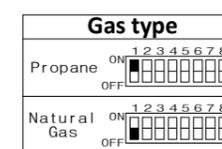
The Gas Type dipswitch should already be properly preset from the factory.
