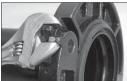
**4a. FOR STYLE 741 AND STYLE 744 FLANGE ADAPTERS ONLY:** Closure lugs are provided for ease of installation. If necessary, use an adjustable wrench to bring the flange holes into alignment. This will ease insertion of the standard flange bolts into the mating holes.
