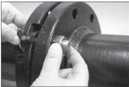
**6a.** Thread standard flange nuts finger-tight onto the two mating bolts.
