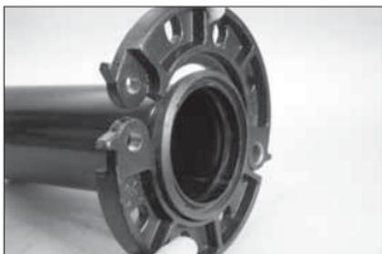
**4. INSTALL FLANGE ADAPTER:** Open the hinged flange adapter fully, and install the flange over the gasket. Make sure the flange key section engages the pipe groove properly.
