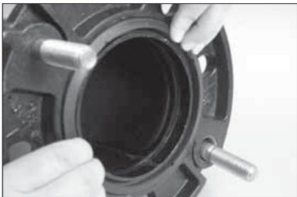
**5a.** Make sure the gasket is seated properly in the flange adapter.
