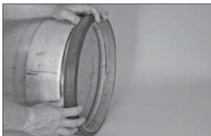
3. **POSITION GASKET:** Position the gasket over the pipe end or AGS Vic-Ring. Make sure the gasket does not overhang the pipe end or AGS Vic-Ring.
