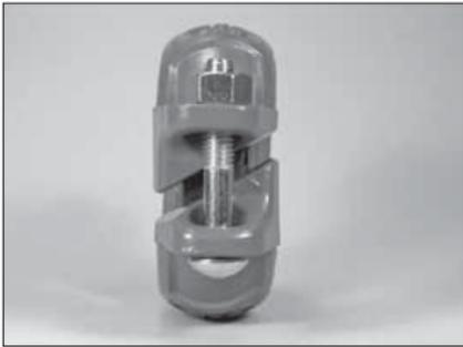
**1. DO NOT DISASSEMBLE THE COUPLING:** Style 107H Couplings are installation ready. The coupling is designed so that the installer does not need to remove the bolts and nuts for installation. This design facilitates installation by allowing the installer to directly install the grooved end of pipe/mating components into the coupling.
