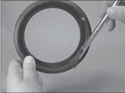
**3. LUBRICATE GASKET:** Apply a thin coat of Victaulic Lubricant or silicone lubricant to the gasket sealing lips and exterior. It is normal for the gasket surface to have a hazy white appearance after it has been in service.
