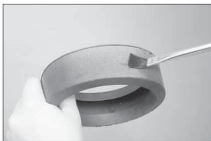
**3. CHECK GASKET AND LUBRICATE:** Check the gasket to make sure it is suitable for the intended service. The color code identifies the gasket grade. Apply a thin coat of Victaulic Lubricant or silicone lubricant to the gasket lips and exterior.
