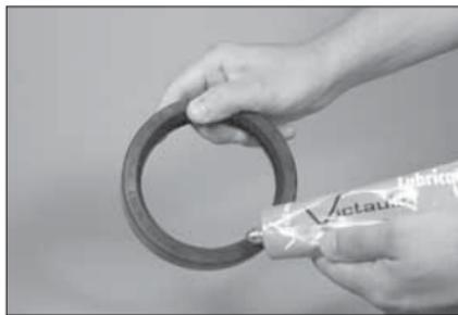
**2. CHECK GASKET AND LUBRICATE:** Check the gasket to make sure it is suitable for the intended service. Apply a thin coat of Victaulic Lubricant or silicone lubricant to the gasket sealing lips and exterior.
