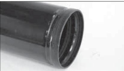
**1. CHECK PIPE ENDS:** The outside surface of the pipe, between the groove and the pipe end, must be smooth and free from indentations, projections (including weld seams), and roll marks to ensure a leak-tight seal. All oil, grease, loose paint, dirt, and cutting particles must be removed.
