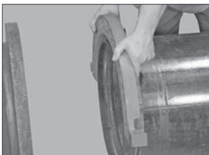
2. **ADD FIRST SEGMENT:** Place the first segment onto the pipe. Make sure the key engages completely in the groove.
