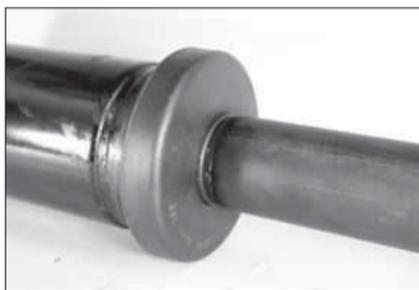
**4. JOIN PIPE ENDS:** Align the centerlines of the pipes and insert the smaller pipe end into the gasket. Make sure no portion of the gasket extends into the pipe groove.
