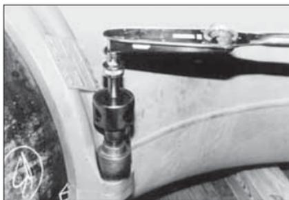
**5. APPLY TORQUE:** Apply 600 ft-lbs/ 814 N•m of torque to each nut with a torque wrench. Due to the high torque requirement, use of a geared torque multiplier is recommended.
