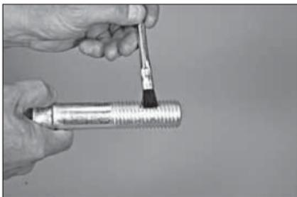
**5. LUBRICATE BOLT THREADS:**
