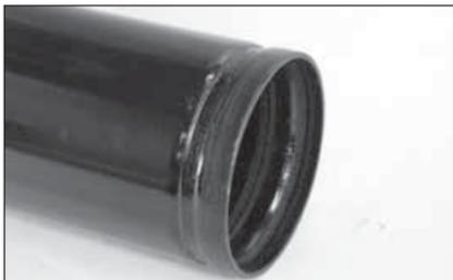
**2. CHECK GASKET AND LUBRICATE:** Check the gasket to make sure it is suitable for the intended service. The Style HP-70ES gasket is molded with a center leg that fits between the pipe ends. Apply a thin coat of Victaulic Lubricant or silicone lubricant to the gasket sealing lips and exterior.
