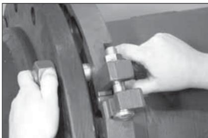
**9. JOIN VIC-FLANGE ADAPTER AND MATING FLANGE:** Direct the four assembly bolts, installed in step 7, into the mating flange holes. Hand-tighten a nut onto each of the four assembly bolts to prevent the bolts from pulling out.
