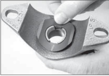
**1. INSTALL GASKET:** Install the gasket into the gasket pocket, as shown above. Press the gasket along the full circumference to ensure that it seats fully in the gasket pocket. **DO NOT LUBRICATE THE GASKET.**
