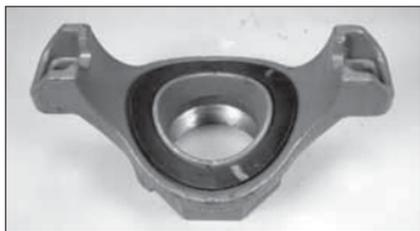
**2. CHECK GASKET AND LUBRICATE:** Inspect the sealing surface of the gasket to make sure no debris is present. For Style 920N Mechanical-T Outlets, it is not necessary to remove the gasket from the housing. **GASKETS FOR THE STYLE 920 ARE NOT INTERCHANGEABLE WITH GASKETS FOR THE STYLE 920N. THE CORRECT GASKET IS SHIPPED WITH THE APPROPRIATE PRODUCT.**
