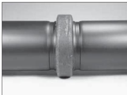
5. **JOIN PIPE/MATING COMPONENTS:** Align the two grooved ends of the pipe/mating components. Insert the other pipe/mating component end into the gasket until it contacts the center leg of the gasket. **NOTE:** Make sure no portion of the gasket extends into the groove of either pipe/mating component.
