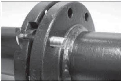
**6. JOIN FLANGE ADAPTER AND MATING FLANGE:** Join the flange adapter with the mating flange by aligning the bolt holes.
