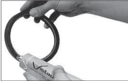
**2. CHECK GASKET AND LUBRICATE:** Check the gasket to make sure it is suitable for the intended service. Apply a thin coat of Victaulic Lubricant or silicone lubricant to the gasket sealing lips and exterior.
