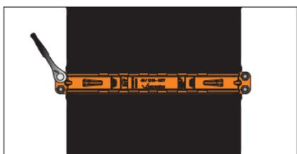
Repeat the tightening sequence shown above until the installation requirements in Step 7 are achieved.
