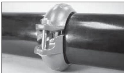
**4. ASSEMBLE JOINT:** Assemble the joint by inserting the grooved end of a pipe/mating component into each opening of the coupling. The ends of the grooved pipe/mating components must be inserted into the coupling until contact with the center leg of the gasket occurs. A visual check is required to ensure the coupling keys align with the grooves in the pipe/mating components. **NOTE:** The coupling may be rotated to ensure the gasket is seated properly.
