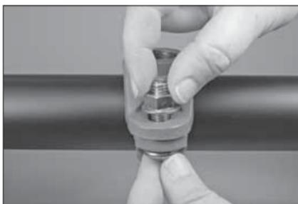
**4. INSTALL REMAINING BOLT/ FLANGE NUT:** Insert the other track bolt into the lower housing and outlet housing. Thread the flange nut onto the bolt finger-tight. Make sure the track heads of the bolts seat properly in the bolt holes.
