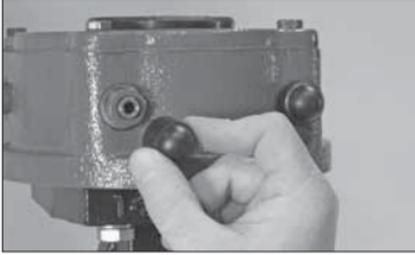
2. Remove the travel stop dust cap from the left side of the gear operator, as shown above.
