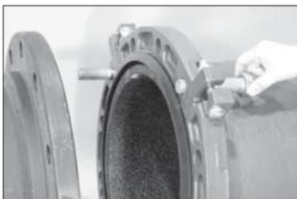
**7. INSERT STANDARD FULL-SHANK DIAMETER ASSEMBLY BOLTS AT LAP JOINTS:** Insert a standard, full-shank diameter assembly bolt into each of the four lap joint holes. **NOTE:** It may be necessary to tighten the draw bolts to line up the lap joint bolt holes for insertion of the bolts.
