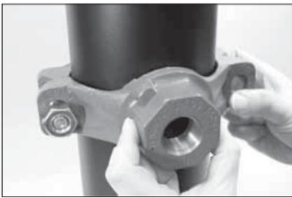
**3a.** Make sure the locating collar engages the outlet hole properly. Check this engagement by rocking the upper (outlet) housing in the hole.
