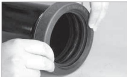
**3. INSTALL GASKET:** Insert the grooved pipe end into the gasket until it contacts the center leg of the gasket.
