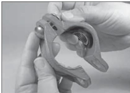
**2. ASSEMBLE HOUSINGS:** Remove the flange nut and bolt from one side of the Style 912 assembly. Thread the remaining flange nut loosely onto the bolt (flange nut should be flush with end of bolt) to allow for the “swing-over” feature.
