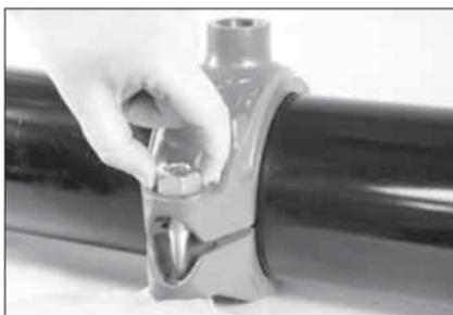
**7. INSTALL BOLTS/NUTS:** Install the bolts, and thread a nut finger-tight onto each bolt. **NOTE:** Make sure the oval neck of each bolt seats properly in the bolt hole.
