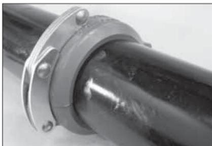
**3a.** Push the locking handle down firmly until the entire handle assembly contacts the coupling housing. The entire handle assembly must contact the coupling housing to ensure a properly locked joint.
