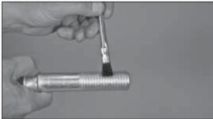
**5. LUBRICATE BOLT THREADS:** Apply a thin coat of Victaulic lubricant or silicone lubricant to the bolt threads. **NOTE:** If stainless steel bolts and nuts are special ordered, apply an anti-seize compound to the bolt threads.
