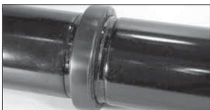
**4. JOIN PIPE ENDS:** Align and bring the two pipe ends together. Insert the other pipe end into the gasket until it contacts the center leg of the gasket. **NOTE:** Make sure no portion of the gasket extends into the groove of either pipe.
