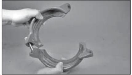
6. **TO FACILITATE RE-ASSEMBLY:** One bolt can be inserted into the housings with the nut threaded loosely onto the bolt to allow for the “swing-over” feature, as shown above. **NOTE:** The nut should be backed off no further than flush with the end of the bolt.
