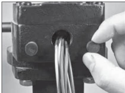
2. Remove the travel stop dust cap from the right side of the gear operator, as shown above.
