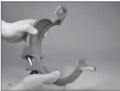
**6. TO FACILITATE RE-ASSEMBLY:** One bolt can be inserted into the housings with the nut threaded loosely onto the bolt to allow for the “swing-over” feature, as shown above. **NOTE:** The nut should be backed off no further than flush with the end of the bolt.
