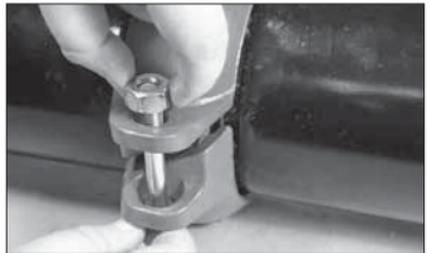
8. **INSTALL REMAINING BOLT/NUT:** Install the remaining bolt, and thread the nut finger-tight onto the bolt. **NOTE:** Make sure the oval neck of each bolt seats properly in the bolt hole.
