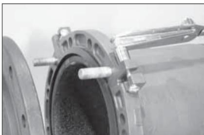
**8. TIGHTEN DRAW BOLTS:** After the four assembly bolts are inserted into the lap-joint bolt holes, torque the draw bolts to approximately 150 ft-lbs/203 N•m. **NOTE:** It is normal to have a small amount of shift as these bolts are being torqued.
