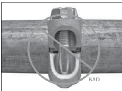
**4. TIGHTEN NUTS:** Tighten all nuts evenly by alternating sides. Make sure the housings' keys engage the grooves completely on both pipe ends. Apply torque to each nut with a torque wrench. Refer to the following table for the torque requirement. **NOTE:** It is important to tighten the nuts evenly to prevent gasket pinching.
