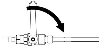
Turn on the main supply valve. Run the filtered water for 2 minutes to flush the system, and carefully check the system for leaks. The system is now ready for use.
