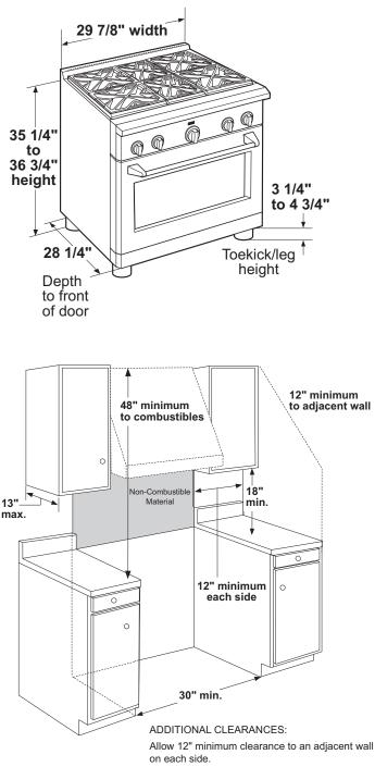
Working areas adjacent to the rangetop should have 18" minimum clearance between countertop and the bottom of the wall cabinet.
