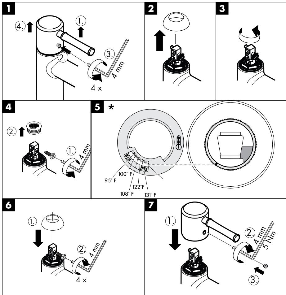
\*The temperatures given in the diagram assume a water heater temperature of 140° F, a cold water temperature of 50° F and a water pressure of 44 PSI.
