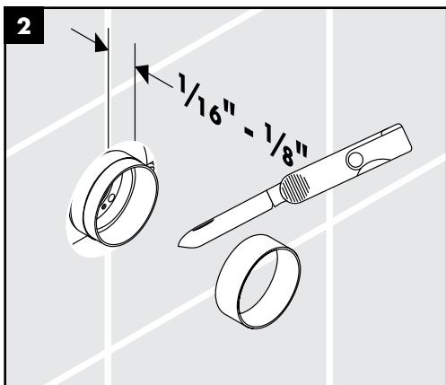
Cut the plaster shield so that it extends  $1/16''$  -  $1/8''$  outside the surface of the finished wall.
