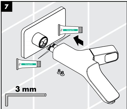
Lightly lubricate the faucet o-rings using white plumbers' grease.
