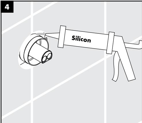
**Seal the wall around the plaster shield with waterproof sealant.**
