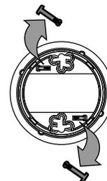
Close Door. Insert Pin in Holes through alarm and Battery Drawer
