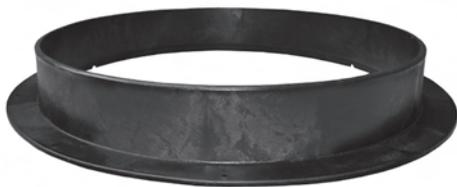
Infiltrator's **Pipe Adapter Ring** provides a watertight connection when using HDPE, IPEX or Ultra Rib pipe with the TW-Series Septic Tanks. The pipe adapter ring has alignment slots, which securely lock onto the alignment tabs located on the reinforcing ring. This provides an ideal connection for watertight performance.
