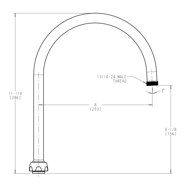
DIMENSIONS ARE IN INCHES AND [MILLIMETERS].
