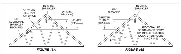
There can be a maximum of a 6 in. (152,4 mm) high Horizontal Obstruction as long as it is 36 in. (914,4 mm), measured vertically, below the Attic Sprinkler. If the obstruction is closer or larger, there must be a sprinkler on the other side of the obstruction. Refer to Figures 16A and 16B. This criteria does not limit the top chord of the trusses or the depth of the rafter, but does limit the obstructions that run across the trusses or rafters.
