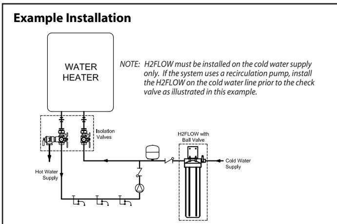
\*The effectiveness of the H2Flow cartridge will depend on the chemistry of the cold water supply. Refer to the Water Chemistry & Limitations chart located above. Changing the H2FC cartridge at least once every **TWO** years is recommended.
