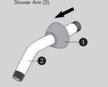
Apply Teflon Tape to inlet side of Shower Arm (2). Thread Shower Arm (2) into Female Pipe Fitting within the wall. Firmly tighten, and make sure Shower Arm (2) Outlet is pointing in a downward position.
