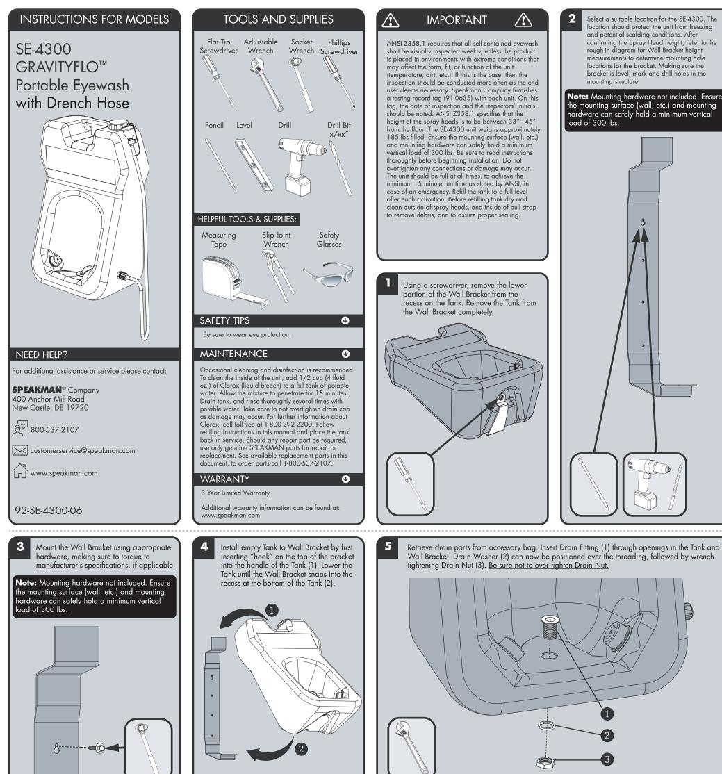
Select a suitable location for the SE-4300. The location should protect the unit from freezing and potential scalding conditions. After confirming the Spray Head height, refer to the rough-in diagram for Wall Bracket height measurements to determine mounting hole locations for the bracket. Making sure the bracket is level, mark and drill holes in the mounting structure.
