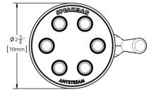
Max. Flow Rate: 2.5 gpm (9.5L/min) Min. Flow Rate: 2.0 gpm (7.6 L/min) @ 45psi FOR USE WITH AUTOMATIC COMPENSATING VALVES RATED AT 7.6 L/MIN (2.0 GPM) OR LESS.
