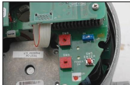
Easily accessible control panel helps allow setting of torque, speed, and position quickly and simply. All settings are done from this control panel.
