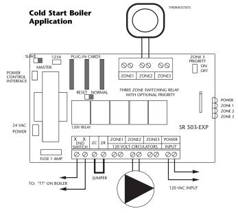
**Operation:** When the thermostat calls for heat, the appropriate circulator is energized and the isolated end switch (X and X) will start the boiler.
