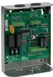
The Hydro Air Fan Control is the ideal interface between the thermostat and air handler. The Fan Control provide advanced diagnostic capabilities, universal thermostat compatibility, a simplified wiring layout, and automatic multi-speed switching. It also includes built-in fan delays, pump and boiler contacts, pump exercise timer, and a secondary aquastat connection for freeze protection.
