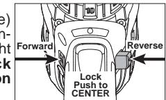
For **forward** (clockwise) rotation, push in the control switch from the right side of the tool. **Check the direction of rotation before use.**
