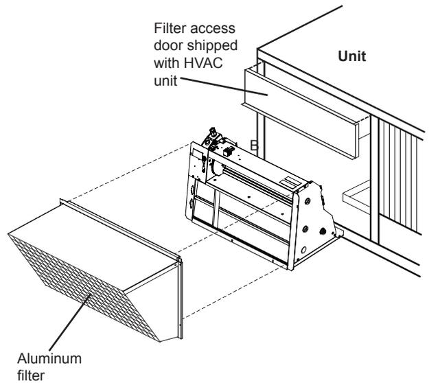
**Fig. 5 - Economizer Installed in HVAC Unit (ECD-SRT12DR Shown)**
