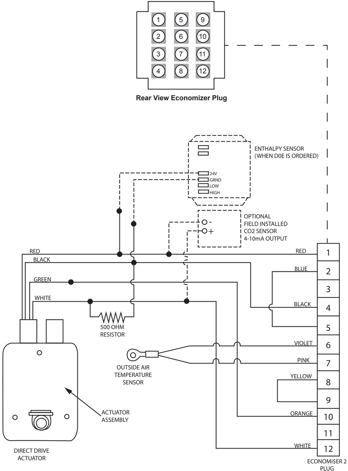
**Fig. 7 - Economizer with No Controller for DDC
