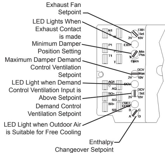
**Fig. 13 - Economizer Controller Potentiometer and LED Locations**
