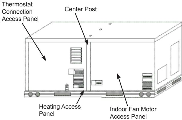
**Fig. 23 - Typical Indoor Fan Motor Access Panel Locations**
