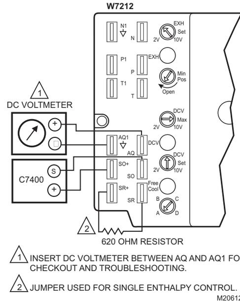
**Fig. 20 - Meter Location for Checkout and Troubleshooting**
