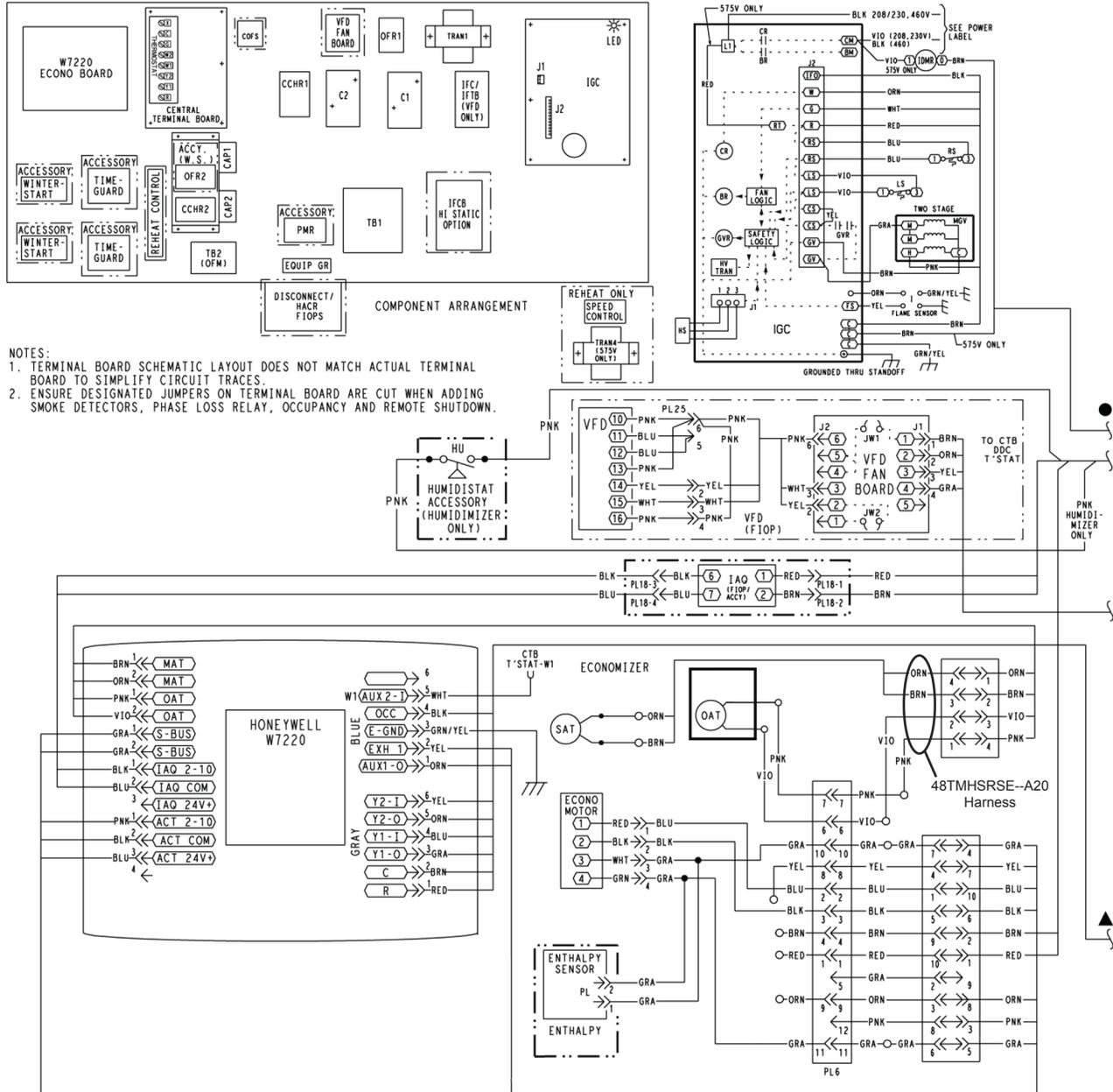
Fig. 21A - Typical Economizer Wiring Diagram For W7220 Controller 1 and 2 Speed Units (Similar to Economi\$er X)
