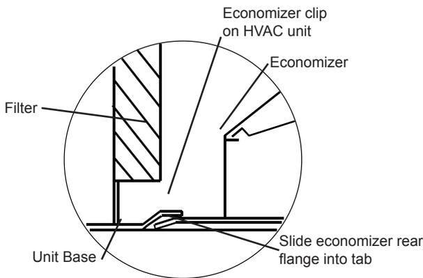
**Fig. 4 - Rear Flange Detail (ECD-SRT12DR and ECD-SRT34DR)**
