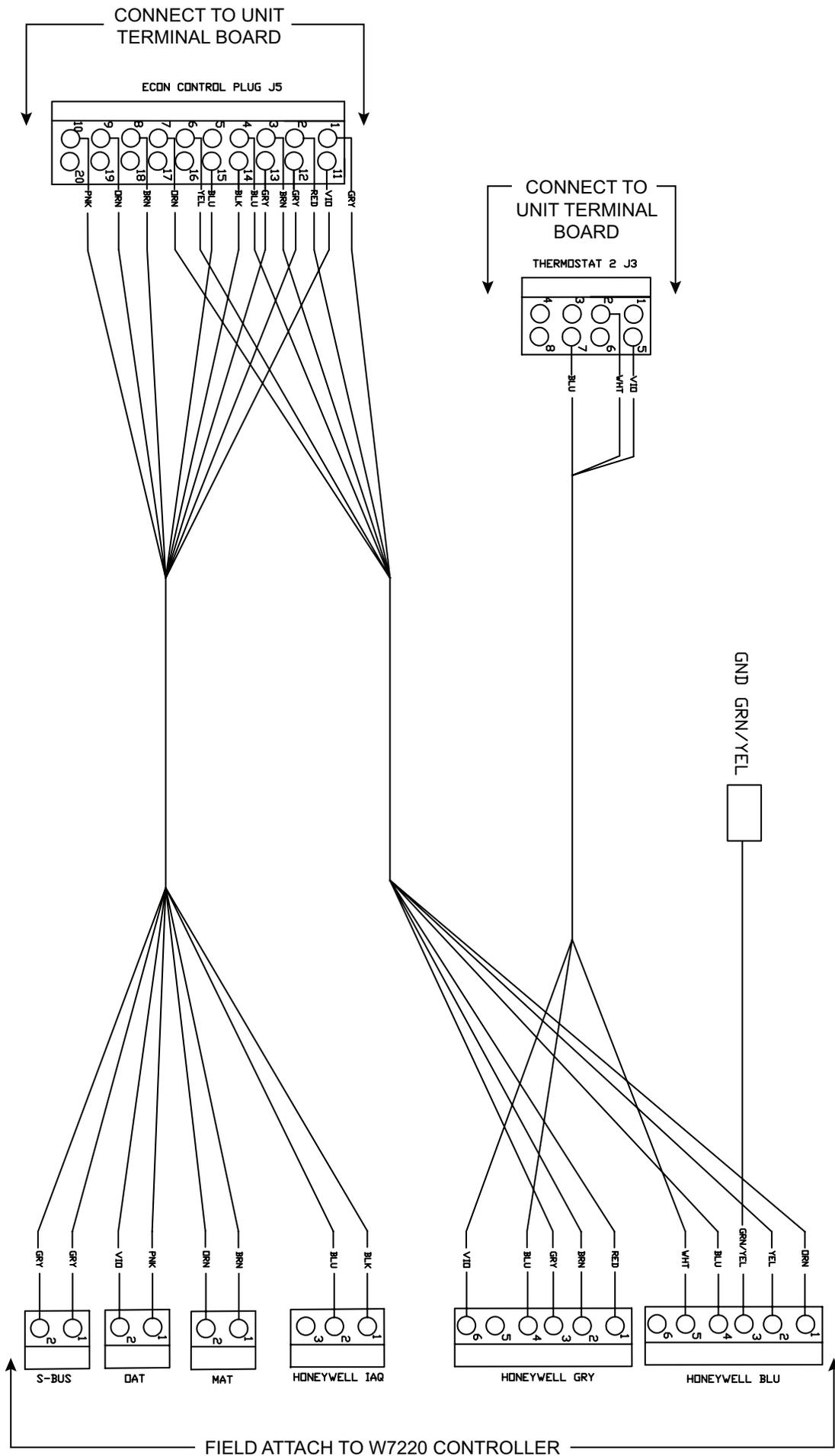
Fig. 21C - 48LCHSRADH--A00 Harness for 3 Speed Units (48/50LC 07-12)
