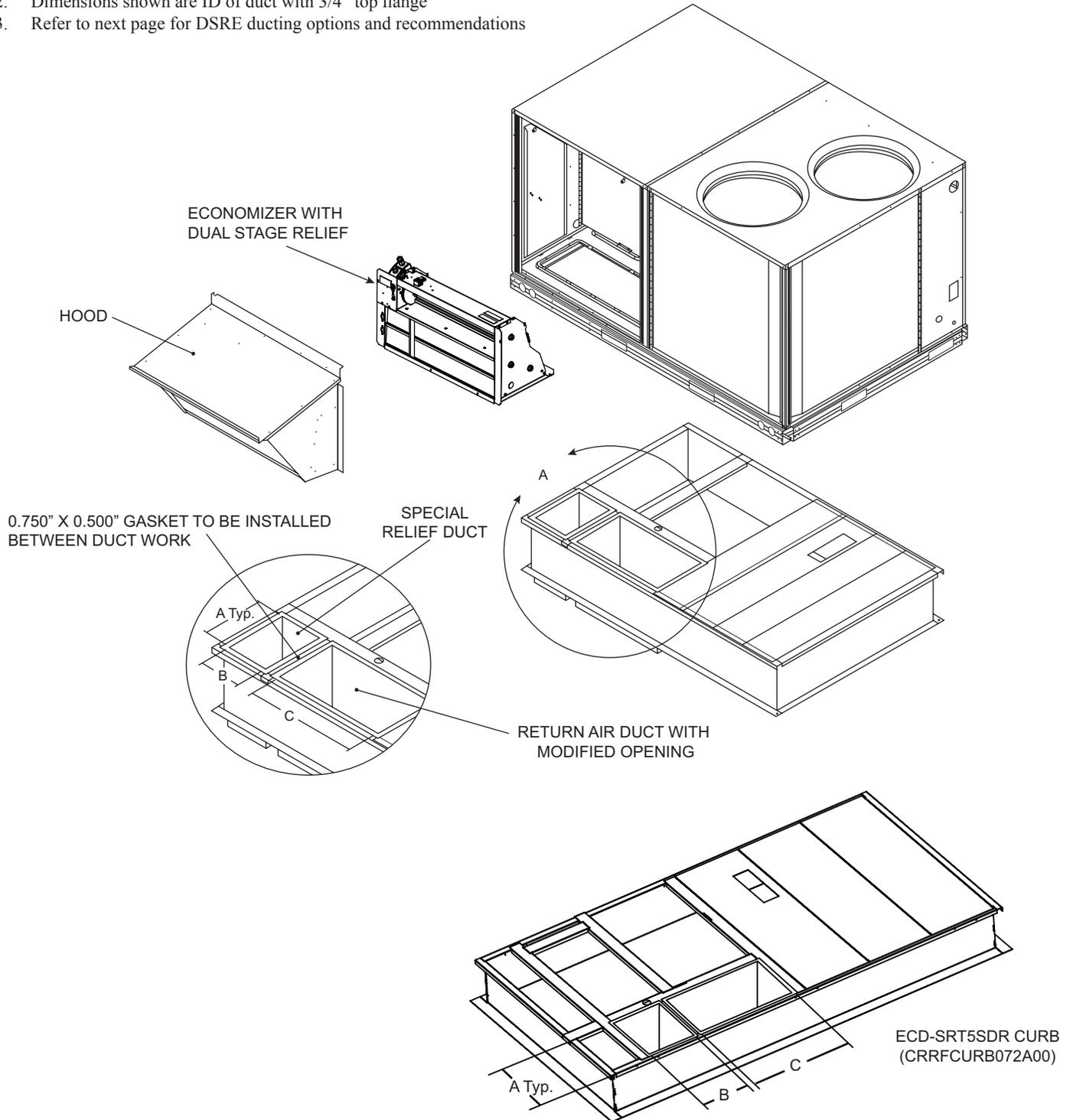
**Fig. 6 - Relief Duct Reference View**
