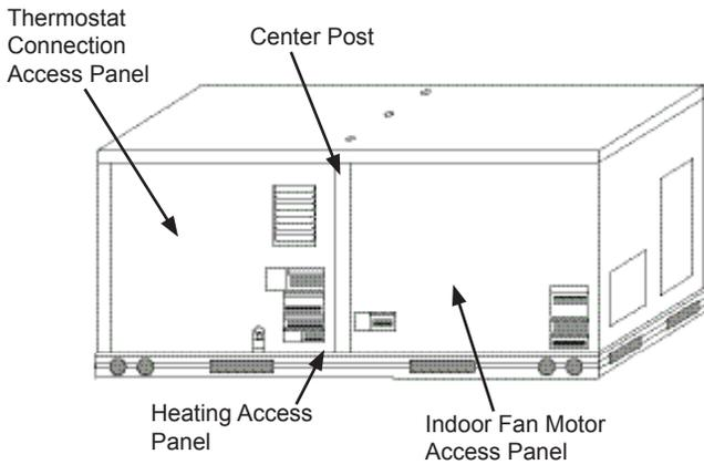
**Fig. 10 - Typical Indoor Fan Motor Access Panel Locations**
