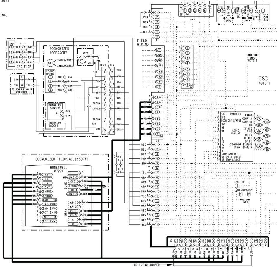
**Fig. 21B - Typical Economizer Wiring Diagram For W7220 Controller 3 Speed Units (48/50LC 07-12)
