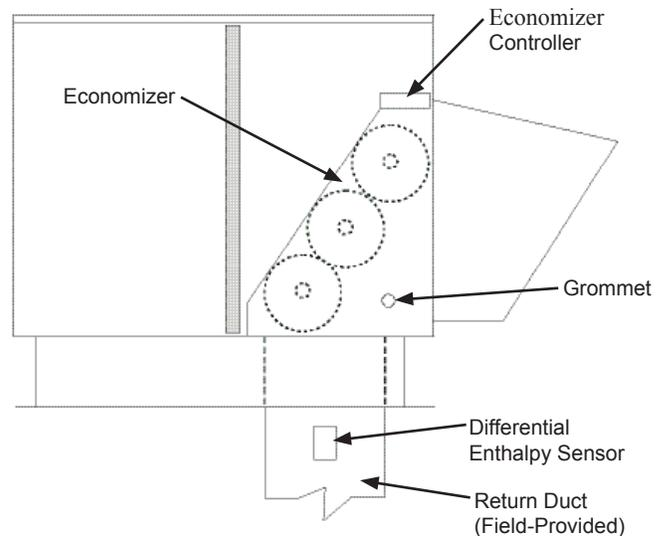
**Fig. 15 - Return Air Enthalpy Sensor Mounting Location**
