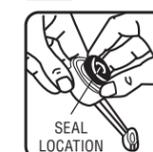
**If Replacing Seal: Use only a genuine Fluidmaster 242 seal.**
