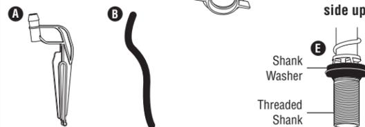
Place shank washer onto threaded shank of fill valve. **Flat side up.**
