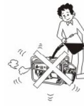
Fill fuel tank outdoors and never overfill the tank.
