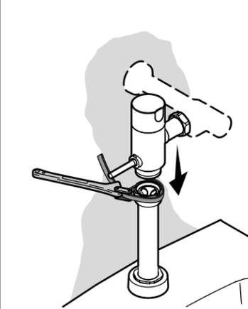
**9** Align and tighten the valve to the control stop.
