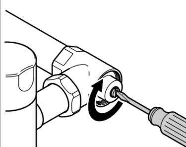
**14** Open the control stop valve 1/4 turn at a time until an adequate flush is achieved. Reinstall the cap.
