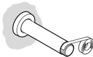
**5** Connect and tighten the control stop to the supply tube. Align the control stop outlet to the valve inlet.
