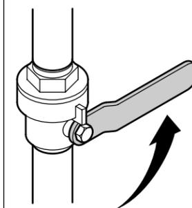
**11** Remove the cap. Turn the screw counterclockwise to fully open the control stop valve.
