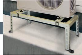
Raises condenser up to 12<sup>1</sup>/<sub>4</sub>" above a flat surface. Each leg is independently adjustable for uneven surfaces. Includes Anti-vibration mounts and anti-slip rubber feet and I
