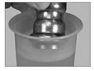
IF PRODUCT IS NOT SHIPPED FROM THE FACTORY IN A BAG, THE SEALS ARE NOT PRE-LUBRICATED AND MUST BE LUBRICATED IN THE FOLLOWING MANNER. Lubrication is essential to prevent seals from being pinched during installation. Fittings should be dipped into a soapy water solution. Make sure the seals are wetted thoroughly, and complete all pressing steps while the
